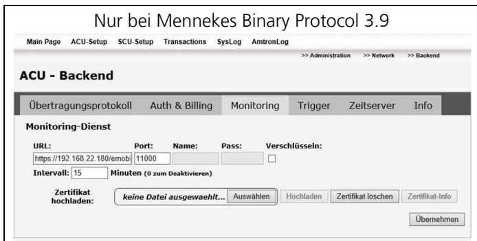
Abb. 20: ACU Backend – Monitoring
