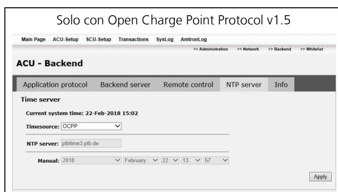
Fig. 23: ACU Backend – NTP server
