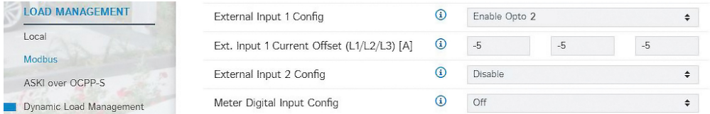
Fig. 39: Web interface of the DLM-Master for configuring the downgrade input of the entire charging point network
